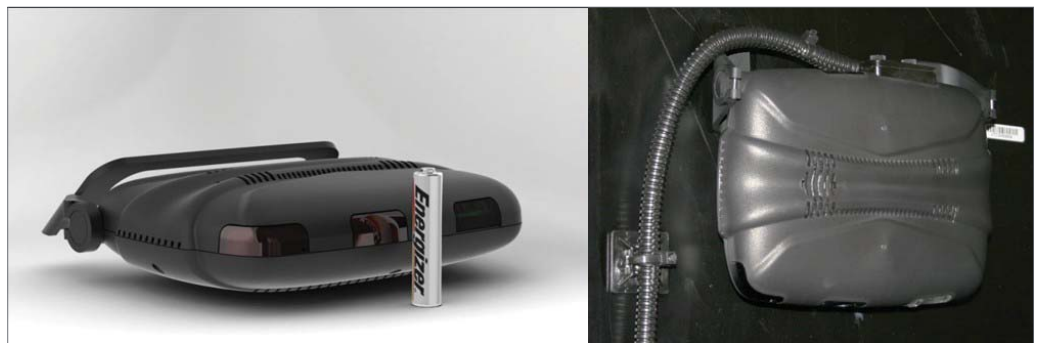
FIGURE 4-2 VTTI MiniDAS VEHICLE DATA-COLLECTION INSTRUMENT WITH AA BATTERY (LEFT) AND MOUNTED ON A BUS (RIGHT)
